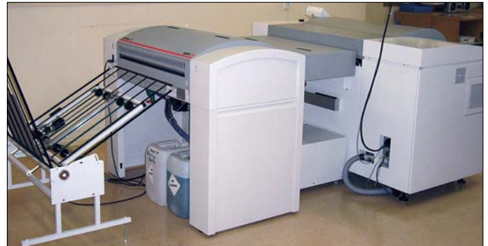
A side view of the :Acento S platesetter (to right) with the :Azura C85 gumming unit at left.
